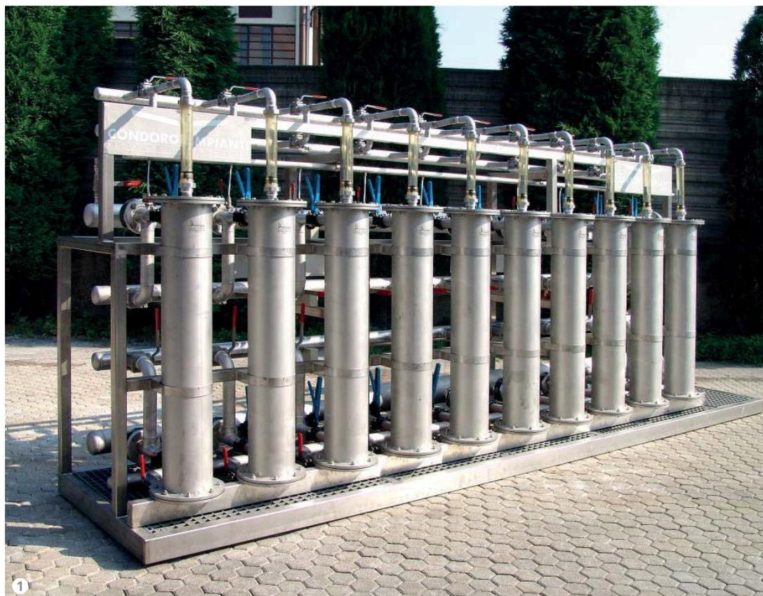
Figure 1: Giunone is the ultrafiltration automatic plant designed by Condoroil Stainless.
